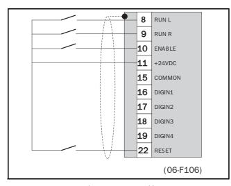
Fig. 26 Wiring example Run/Stop/Enable/Reset inputs
