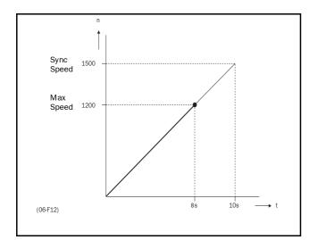
Fig. 40 Acceleration time and maximum speed.
