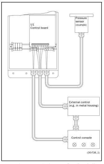
Fig. 14 Electro Magnetic (EM) screening of control signal cables.
