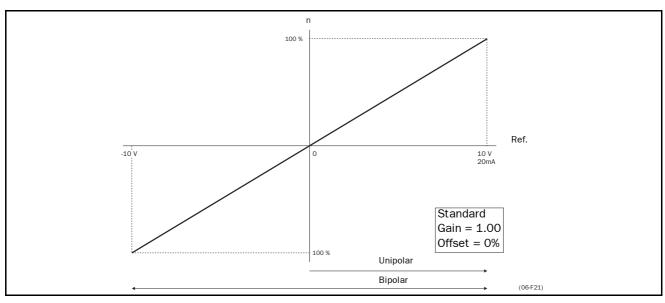
Fig. 54 Normal full-scale configuration.
