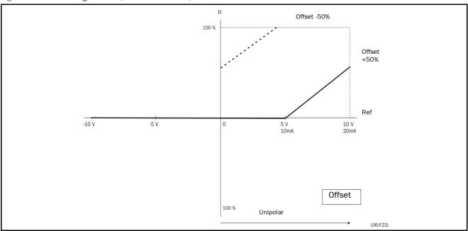
Fig. 56 Function of the Offset setting.
