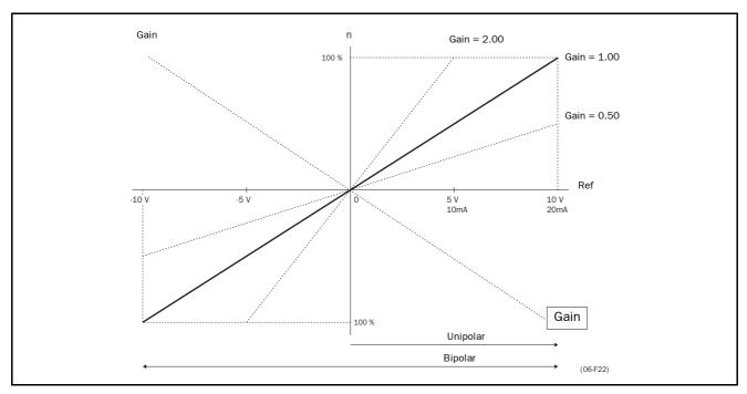
Fig. 57 Function of the Gain setting.
