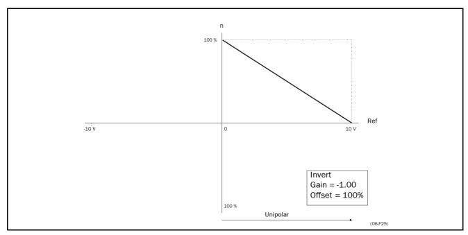
Fig. 58 Inverted reference
