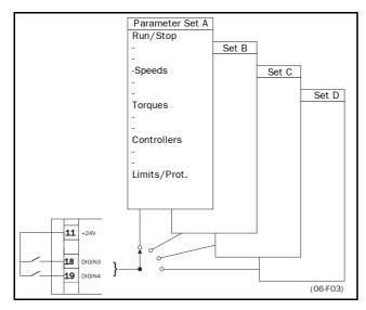
Fig. 31 Selecting the Parameter Sets.
