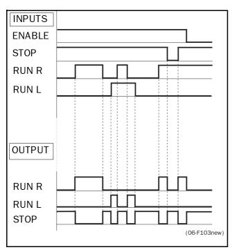
Fig. 29 Run/Stop/Enable functions Level-controlled.
