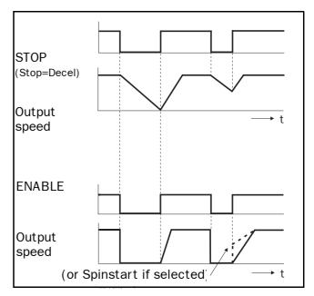
Fig. 27 Functionality of the Stop and Enable input.
