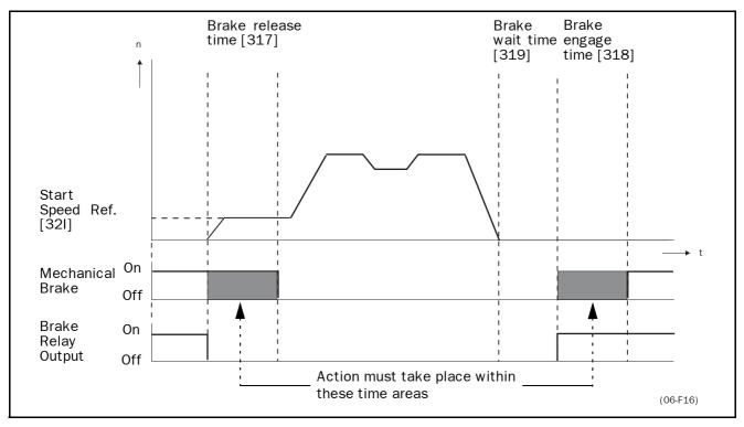
Fig. 44 Brake Output functions.
