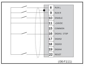
Fig. 28 Wiring example Run/Stop/Enable/Reset inputs.
