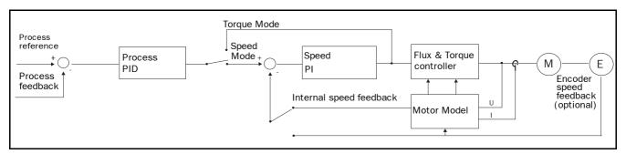
Fig. 51 Closed loop PID control.
