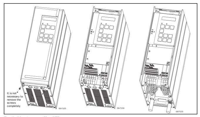
Fig. 12 Mounting power cables - VFB
