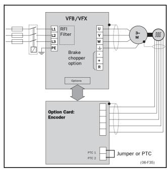
Fig. 75 ENCODER card connection.
