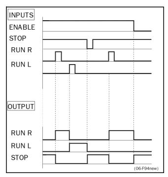
Fig. 30 Run/Stop/Enable functions Edge-controlled.
