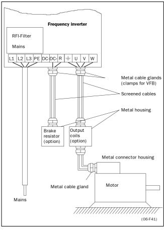
Fig. 8 Frequency inverter as stand alone.
