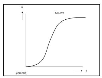
Fig. 42 S-curve acceleration ramp.
