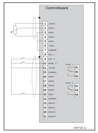
Fig. 2 Minimum control wiring.
