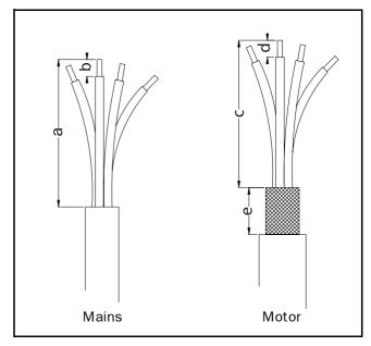
Fig. 11 Stripping lengths for cables - VFX.
