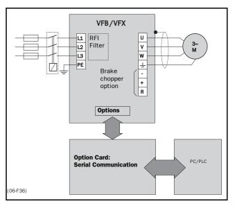
Fig. 76 Connection of a serial link.
