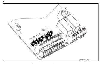
Fig. 16 Location of connectors and jumpers.
