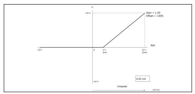
Fig. 55 Gain=1.25 Offset 20% (Live Zero 4-20mA).
