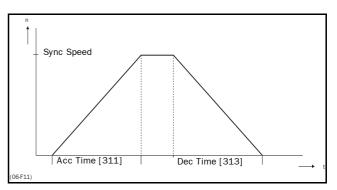
Fig. 41 Acceleration and deceleration times.
