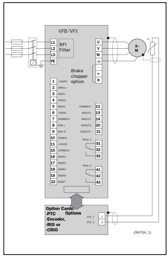
Fig. 74 Connection of the motor thermistor (PTC).
