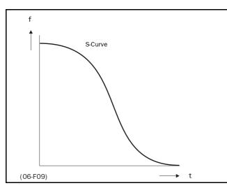
Fig. 43 S-curve deceleration ramp.
