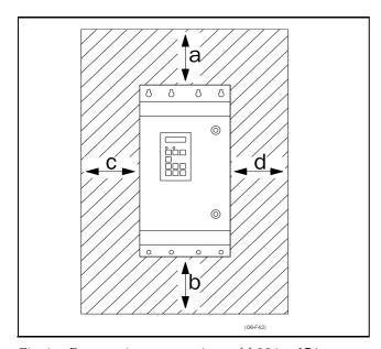
Fig. 4 Frequency inverter mounting model 004 to 374
