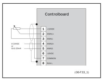
Fig. 3 Using differential inputs.
