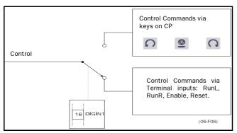
Fig. 37 Run/stp Control = Rem/DigIn 1.
