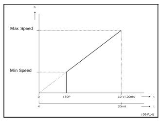
Fig. 48 Min Speed Mode = Stop.
