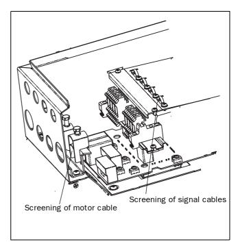
Fig. 9 Screening of cables with size S2.
