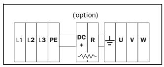
Fig. 6 Mains and motor connection for model 046 to 749.
