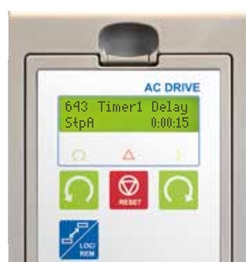
Built-in programming blocks such as timers and comparators allow you to customize functionality.
