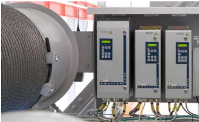
*The IP54 enclosure allowed the variable speed drives to be installed on the crane bridges and the winch. This reduced installation costs.*
