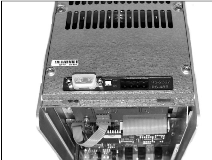
Fig. 6 Mounting of the option card seen from the top.
