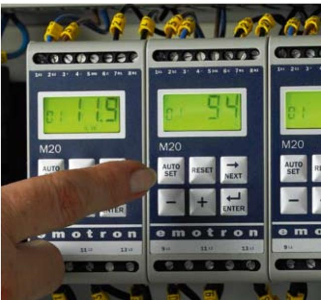
The unique auto-set feature of the Emotron M20 monitor establishes four protection set points in three seconds with just the push of a button.
